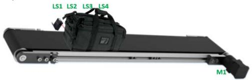
When the 4<sup>th</sup> proximity sensor is activated, if all sensors (LS1, LS2 & LS3) are detecting, this means an over-length luggage is in the sorting belt and the following will occur:
