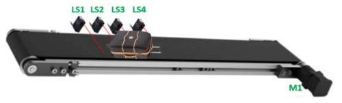
When the 4<sup>th</sup> proximity sensor is activated, if only the 2<sup>nd</sup> and 3<sup>rd</sup> sensor LS2 & LS3) are detecting, this means a Regular luggage is in the sorting belt and the following will occur:
