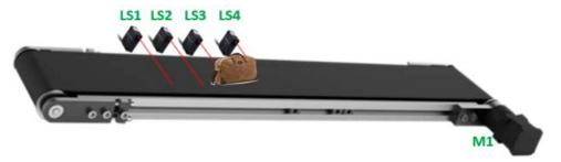
When the 4<sup>th</sup> proximity sensor is activated, if only the 3<sup>rd</sup> sensor (LS3) is detecting, this means a small luggage is in the sorting belt and the following will occur:
