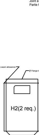
Flange in to match roof curve
