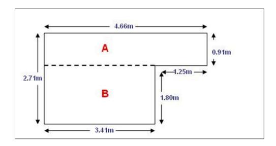
Tile setters calculate area to determine the number of tiles required to complete a floor. Check out the skills tile setters need here.
