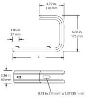
The "J" bracket with TabLok™ profile provides a secure attachment surface requiring no additional hardware for mounting ExpressTray® to ceilings. This bracket is available in 6 in., 8 in., 10 in. and 14 in. lengths to accommodate wire basket profiles up to 12 in. wide and 4 in. high. Available in pregalvanized steel.
