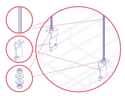
Another method of ceiling-mounted support, side hangers (see page C25) are an alternative for tray that cannot be supported using the center-hung clamp. 1/4 in. threaded rod (see page C26) is threaded into side hangers, the tray is hooked onto the hangers and pivoted into position. Tray is held securely in position by means of a set screw which prevents the wire from jumping out of the side hanger.
