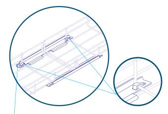
As the name suggests, the Quick Splice shown on page C14 is another quick method for attaching straight sections of ExpressTray® together.
