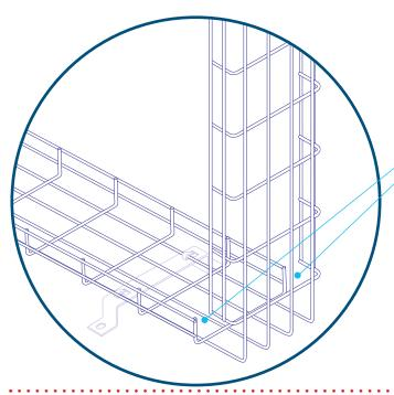
To create a  $90^\circ$  vertical bend, remove one section of side wires on each side of the tray at the point where the angle is required and bend into position.
