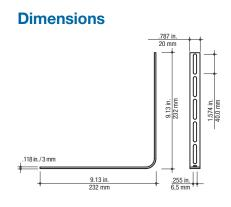
Create high strength tee, cross and other 90 degree configurations with this 90 degree bracket. Available in hot-dipped galvanized steel either as a single bracket or a kit including one (1) bracket, four (4) bracket clamps and one (1) hot-dipped galvanized universal splice.
