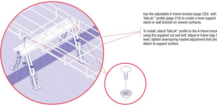
To install, attach TabLok™ profile to the A-frame bracket using the supplied nut and bolt. Adjust A-frame legs to level, tighten downspring-loaded adjustment bolt and attach to support surface.
