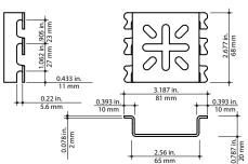
These versatile mounting bases can be used as a wall mount attachment, as a support for electrical outlet boxes and as an under floor attachment. Quick and easy to install, tray mounts securely to the base using fold-over tab attachments. No additional hardware is required. The small mounting base is available in hot-dipped galvanized steel and stainless steel (Type 316) and can be used for tray widths from 4 in. to 24 in.
