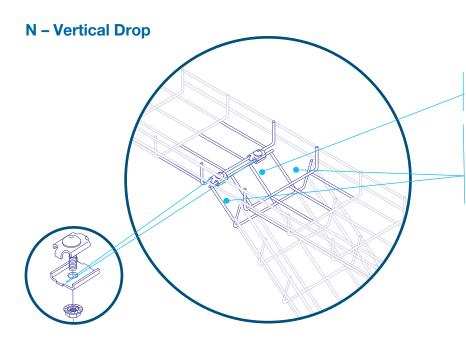
To redirect select cables from a main run, cut and remove bottom wires of tray in accordance with space required for tray intersection.
