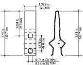
The under-floor support clamp attaches to round and square floor posts and is used to support TabLok $^{\text{\tiny M}}$  profiles in under floor applications. Available in pregalvanized steel, the under-floor clamp is supplied with all necessary hardware.
