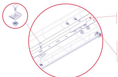
For separating bundles of power, voice and data cables, barrier strips (see page C27) can be attached along the length of the tray bottom.
