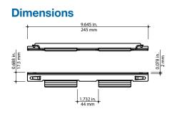
Connect straight lengths up to 24 in. wide using only two quick splices - no other components required. Simply bend tabs down and lock into position using pliers. Compatible with all profiles, the Quick Splice is available in pregalvanized steel, hot-dipped galvanized steel and stainless steel (Type 316).
