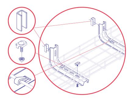
Two types of "L" brackets are available for wall-mounted supports: the standard "L" bracket and the TabLok "L" bracket.
