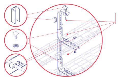
Use brackets to create multi-level installations for applications that require separation of different types of cables.
