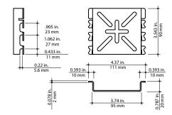
These versatile mounting bases can be used as a wall mount attachment, as a support for electrical outlet boxes and as an under floor attachment. Quick and easy to install, tray mounts securely to the base using fold-over tab attachments. No additional hardware is required. The large mounting base is available in hot-dipped galvanized steel and stainless steel (Type 316) and can be used for tray widths from 4 in. to 24 in.
