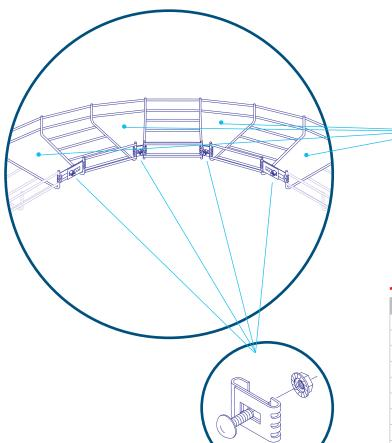
ExpressTray® allows you to redirect cabling routing simply and easily. To form a horizontal bend with a radius, no additional corner or elbow components are required.
