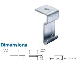
The side hanger clamp is used to construct trapeze supports using threaded rods. The offset support hole allows for trouble-free access to support nuts for height adjustment and the rod can continue downward to allow for multi-level (tiered) trapeze installations. A set screw holds tray firmly in position once installation is complete. Available in pregalvanized steel. For use with 3/8 in. threaded rod.
