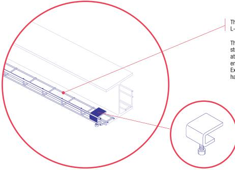
The beam clamp (see page C31) is used to attach L-profile ExpressTray® to steel beams and girders.
