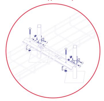
support clamps and secure the profile to the clamp by inserting the supplied bolt through the TabLok™ profile and securing with a nut.
