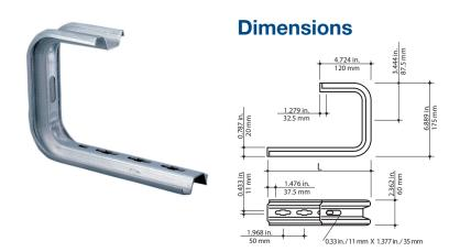
The «J» bracket provides an attachment surface for mounting ExpressTray® to ceilings. This bracket is available in 6 in., 10 in. and 14 in. lengths to accommodate U- and C-profiles of up to 12 in. wide and 4 in. high. Available in pregalvanized steel.
