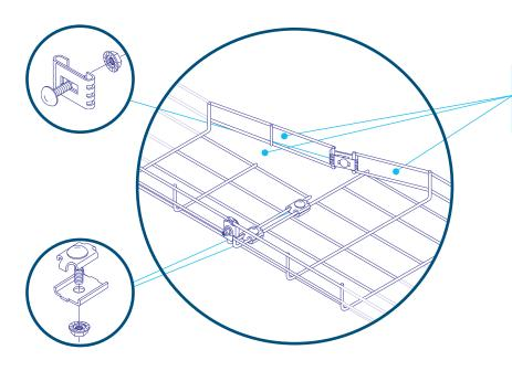
To make the most efficient and economical use of space, it is often necessary to make reductions and expansions of tray widths. To connect two unequal widths of ExpressTray®, a combination of side and bottom wires must be cut and removed.
