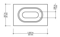
The barrier strip clamp is used to mount barrier strips to ExpressTray® profiles. Available in electrogalvanized steel, hot-dipped galvanized steel and stainless steel (304 and 316).
