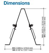
The adjustable A-frame bracket can be used in conjunction with TabLok  $^{TM}$  profile to create support stands or wall brackets for use on uneven surfaces. Bracket is fully adjustable — height varies from 5 to 8 in. — and is available in pregalvanized steel.
