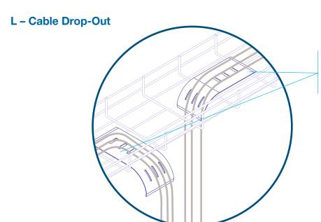
To ease the strain on cables when exiting or entering runs of ExpressTray®, install this 2 in. radius cable drop-out (see page C24). Quick and easy to install, this cable drop-out attaches to tray using built-in tabs. It can also be used as a radius limiter on tees, crosses and vertical bends.
