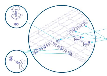
To create a horizontal 90° tee junction without a radius from two straight sections of ExpressTray®, use the 90° brackets shown on page C23.
