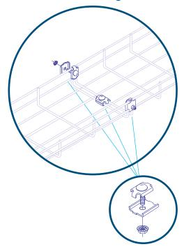
The Universal Splice shown on page C14 can also be used to attach straight sections of ExpressTray® together. Align the two lengths of tray and attach using Universal Splices on top siderail wires and tray bottoms.
