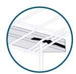
Position "BAT" Clip on outer wires of tray and opposing sides of the strut flanges
