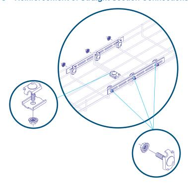
Use two reinforcing Splice Bars (see page C15) to reinforce the connection of any two straight lengths of wire basket tray. To install, center the splice bar over the tray connection on one side of tray and attach to tray side rail using bracket clamps (see page C33). Repeat process to secure to opposite side of tray.
