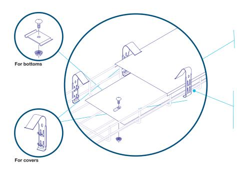
For environments where cables need protection from dirt build-up or cable damage, install ExpressTray® covers and bottoms.
