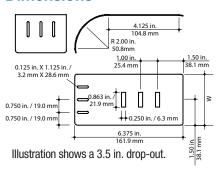
This 2 in. radius cable drop-out protects cables when exiting or entering tray by reducing the strain on the cables. The drop-out attaches to tray with built-in tabs. No hardware is required. Three different widths available in pregalvanized steel. This drop-out is suitable for use with all tray widths and heights.
