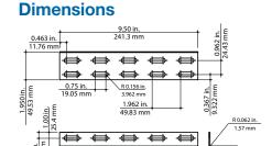
Support and terminate runs of cable tray with this wall termination angle. Can be used as a wall support, floor to ceiling support or to safely terminate any tray run. Adapts to any configuration and any width. Available in pregalvanized steel. Mounting hardware sold separately.
