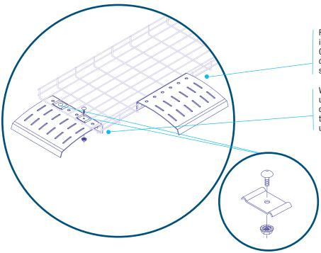
For larger cable tray widths or heavier loads of cables, install the large, 7 in. radius cable drop-out (see page C24) to ease the strain on cables as they exit or enter runs of wire basket tray. The large cable drop-out is ideally suited for use with Category 5 and fiber optic cables.
