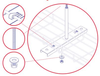
Center-hung configurations are quick and easy when you use the pre-assembled TabLok $^{\text{TM}}$  center-hung assembly. Lock tray into position on the TabLok $^{\text{TM}}$  profile and secure a single 3/8 in. diameter threaded rod (page C26) to the TabLok $^{\text{TM}}$  center-hung assembly using a nut and washer (page C32).
