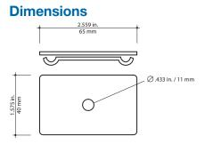
This clamp is used for center-hung applications to secure tray sections to threaded rod for ceiling mounting and can be used with U-profile tray in 4 in., 8 in. and 12 in. widths. This clamp is not designed for use with C-profile tray. Available in pregalvanized steel, hot-dipped galvanized steel and stainless steel (Type 316). For use with 3/8 in. threaded rod.
