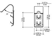
Secure covers to tray quickly with this cover clip. Available in stainless steel (type 301), the cover clip uses built-in tabs to secure the cover and to facilitate removal of the cover when required. No tools required.
