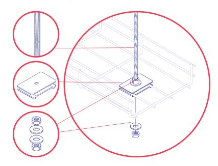
For light-duty applications using 4 in., 8 in. or 12 in. U-profile ExpressTray®, a ceiling-mounted support made up of a single 3/8 in. diameter threaded rod (see page C26) and a threaded rod clamp (see page C26) can be used.The clamp attaches to tray mid-wires as illustrated. A nut and washer (see page C32) are secured on either side of the threaded rod attachment. Order nut and washer separately.
