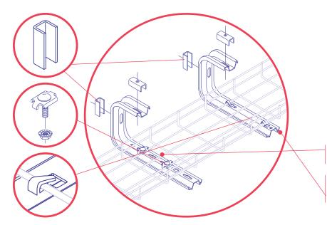
Two types of "J" brackets are available – standard "J" brackets (page C19) and TabLok<sup>TM</sup> profile "J" brackets (page C18).
