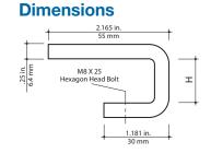
This clamp is used primarily to attach L-profile ExpressTray® to steel beams. It can also be used to attach U- and C-profiles onto structural steel. Available in 3/4 in. and 1-1/8 in. sizes in hot-dipped galvanized steel.
