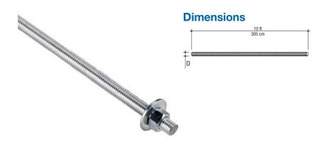
Used for overhead mounting of ExpressTray® with threaded rod clamp, side hanger clamps or strut. Available in 1/4 in. and 3/8 in. diameters, threaded rods are made of electro-galvanized steel.
