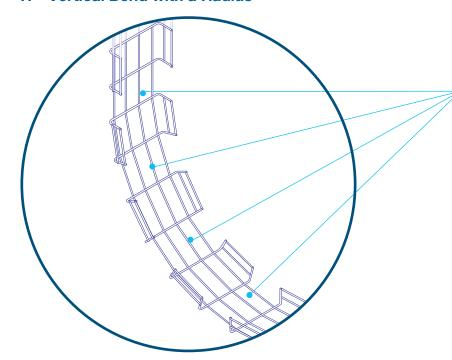
Changing levels using vertical inside and outside bends is easy with ExpressTray®. Simply cut and remove side wires and form to desired bend radius — it's that easy. No additional hardware is required.
