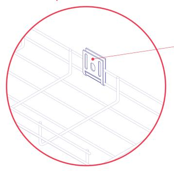
Use wall clamps (see page C25) to attach the side rail of ExpressTray® U- and C-profiles directly to the wall surface. Use standard 3/8 in. hardware to attach (not included).
