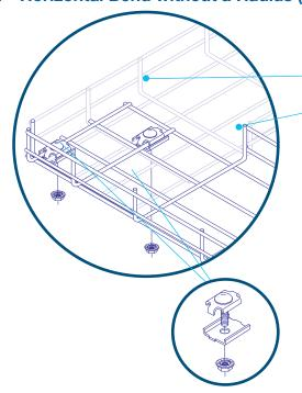
To form a 90° bend or an angled bend without a radius, use two straight sections of tray. Cut and remove side wires (cut back to first complete grid). The number of wires to cut will vary according to the tray width.
