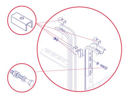
Brackets can be used in a variety of configurations for both wall and ceiling mounting. Attach the bracket profiles together using the back-to-back bracket bolting kit and spacers (see page C34) to prevent distortion of the bracket profile during tightening.
