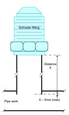
The high-pressure sensing point must be installed as per primary refrigerant flow circuit, and must sense discharge pressure at all times. The sensing point must be located in the discharge line between the compressor and the condenser and located as per supplied drawing and/or demo trainer, if supplied. Only approved fittings shall be used.
