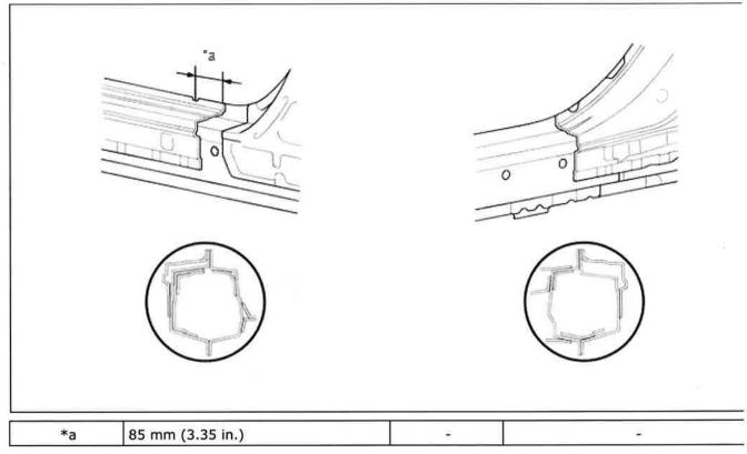
(d) Roughly cut open the panel so that the adhesive can be reached. Cut through the adhesive with a cut c to remove the panel.
