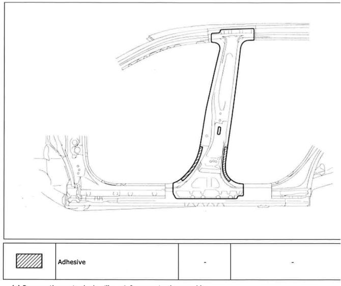
(e) Remove the center body pillar reinforcement sub-assembly.
