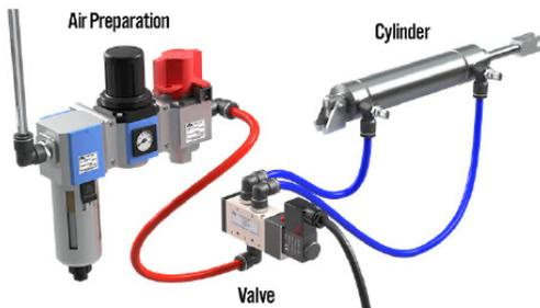
Figure 1C : Basic pneumatic system
