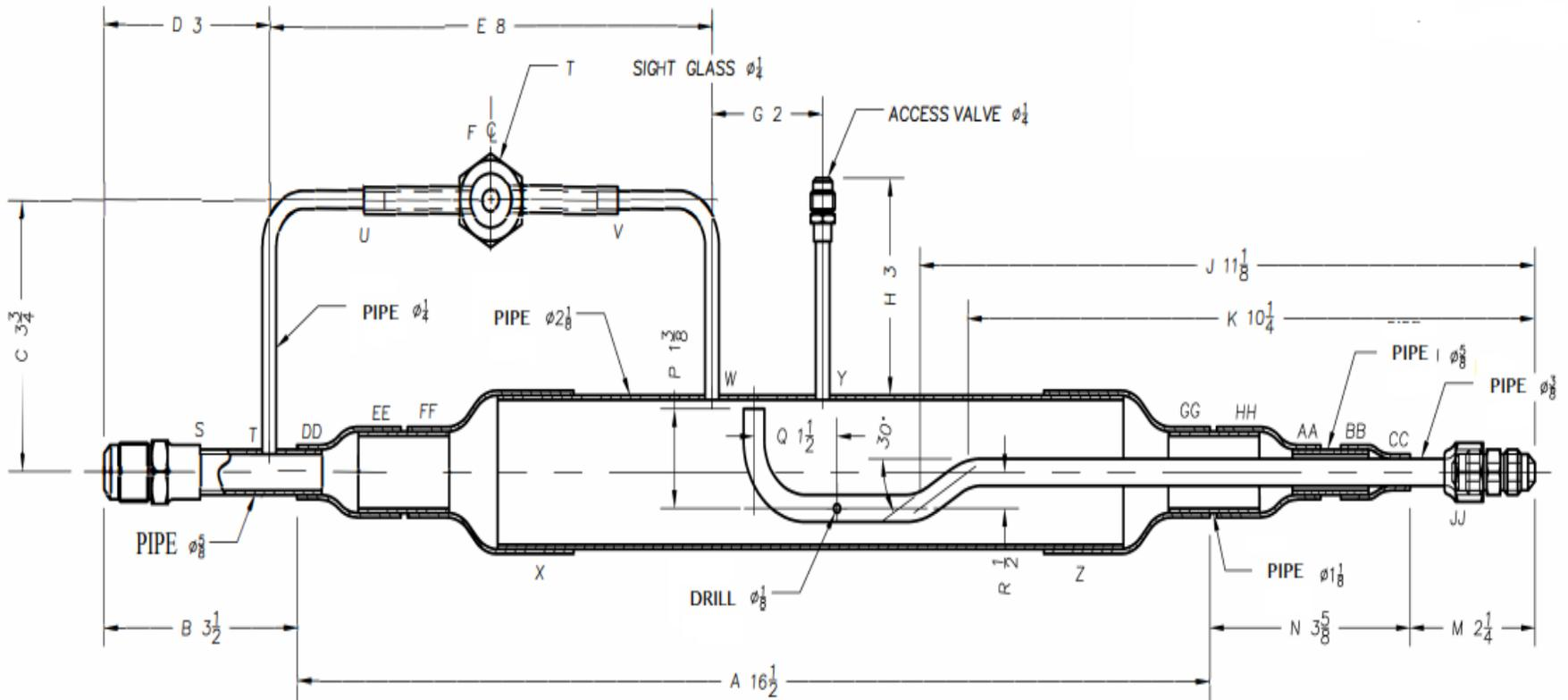
ALL PIPES PASSING THRU A HOLE ARE LEVEL WITH THE WALL OF THE PIPE TO WHICH THEY ARE BRAZED +/- 1/8"
