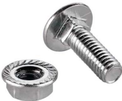
The standard bolting kit consists of an M6 x 12mm carriage bolt and capture nut. Available in electro-galvanized steel, hot-dipped galvanized steel and stainless steel (304 and 316).
