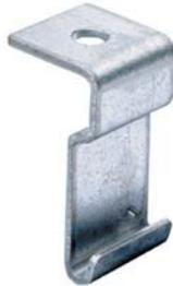
The side hanger clamp is used to construct trapeze supports using threaded rods. The offset support hole allows for trouble-free access to support nuts for height adjustment and the rod can continue downward to allow for multi-level (tiered) trapeze installations. A set screw holds tray firmly in position once installation is complete. Available in pregalvanized steel. For use with 3/8 in. threaded rod.
